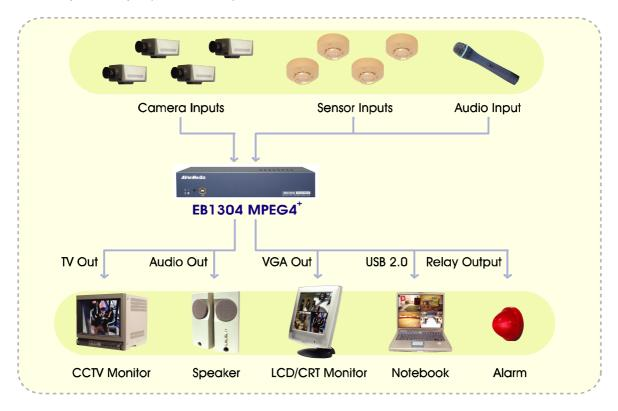
Connecting cameras, sensors, alarm, and display device
